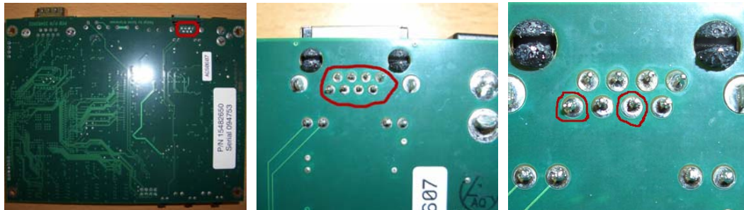
Figure 5: The location of the ethernet jack pins on the bottom of the Soekris net4826 board. The image on the top left shows the whole board, the image on the top right is a close up shot of the ethernet jack pins, and the image on the bottom identifies the particular pins in question. The interesting parts of all images are circled.
