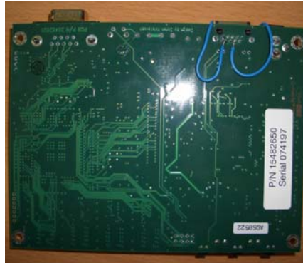
Figure 6: The wires soldered to the ethernet jack pins on the bottom of the Soekris net4826 board.
