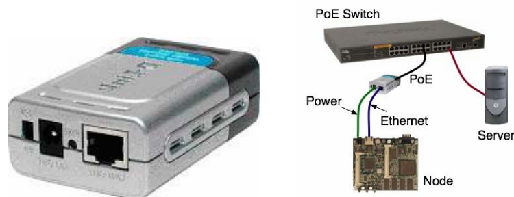
Figure 1: D-Link DWL-P50 PoE adapter and use of PoE adapter
