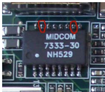
Figure 3: The location of the center tap pins for the Ethernet isolation transformer on the Soekris net4826 board. Each of the two pins is circled.
